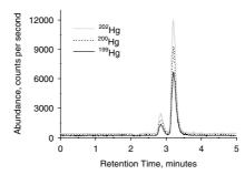
The determination of methylmercury in biological samples by HPLC coupled to ICP-MS detection
